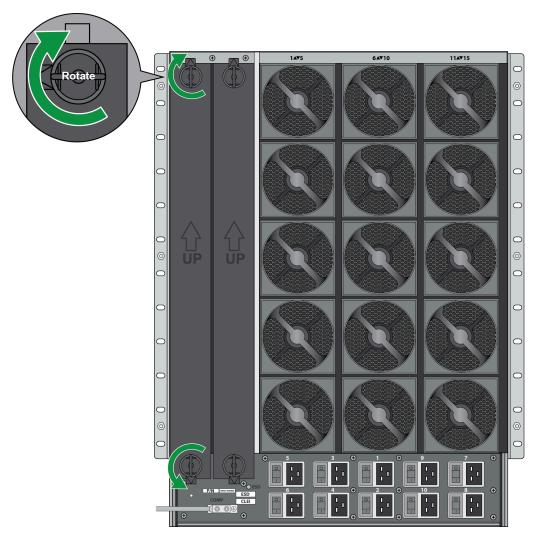
To remove the blank, turn the thumb tabs so that it is unlocked from the chassis. Pull the blank outwards.
