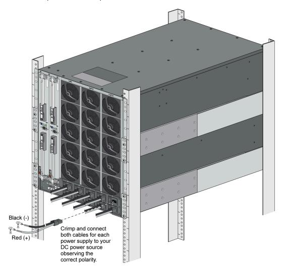
STEP 8 | Connect the other ends of the DC cables to the front of the DC power supplies by pushing the plastic connector into the DC power supply until it clicks into place.
