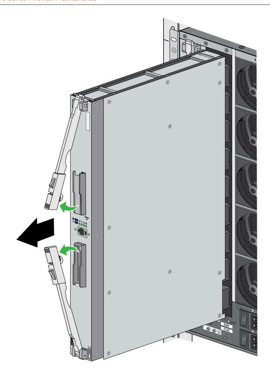
**STEP 4** | Grip the ejector handles and gently pull the card out of its slot.
