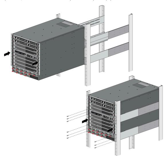
STEP 8 | Use the provided 8-32 x 3/8" Phillips panhead screws to secure the back side of the PA-7500 to the previously mounted brackets.
