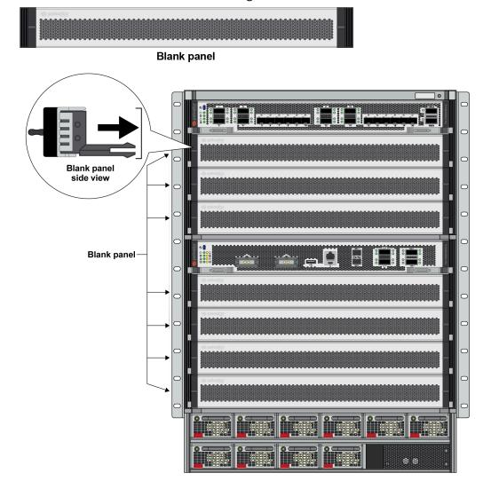
To remove the blank, grip the two handles and pull it outwards. Some force may be necessary to remove the blank.
