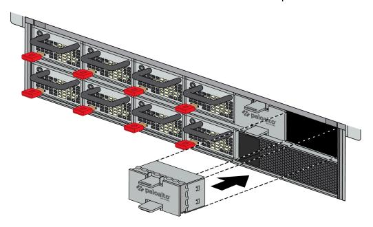
To remove the blanks, press the thumb tabs towards each other and then pull the blank outwards.
