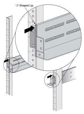
STEP 2 | Position the bottom edges of the fixed and adjustable brackets to the bottom of the 14 RU rack space reserved for the PA-7500. Align the slotted holes of the fixed mounting bracket
