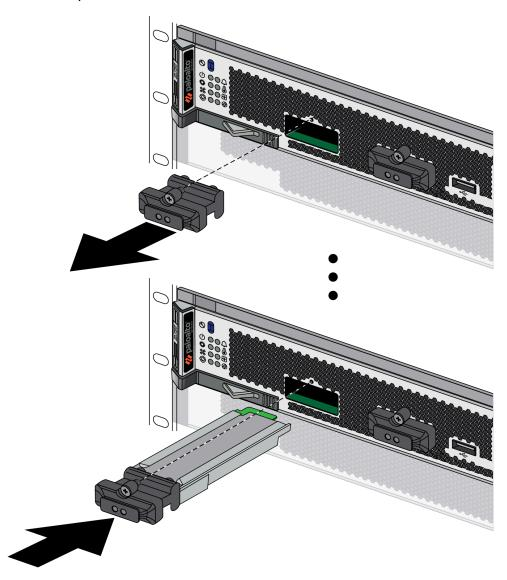
**STEP 7** Once the logging drive is fully seated, tighten the retainer screw to 4 in-lbs.
