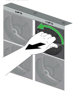
STEP 5 | Install the replacement fan by sliding it into the vacant fan slot. Turn the handle to the right to secure the fan assembly in place.
