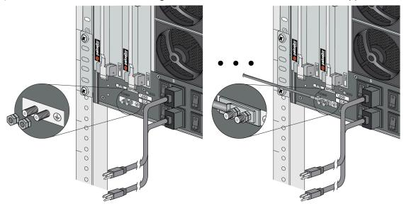
STEP 4 | Crimp a 6-AWG wire to the provided grounding lug and connect the other end to your earth ground point.
