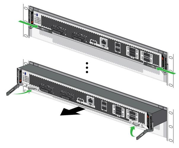
• (SFC) Push the ejector tabs on the card away from the center, prompting a click. This will allow the ejector handles to rotate outward and unlock the card.
