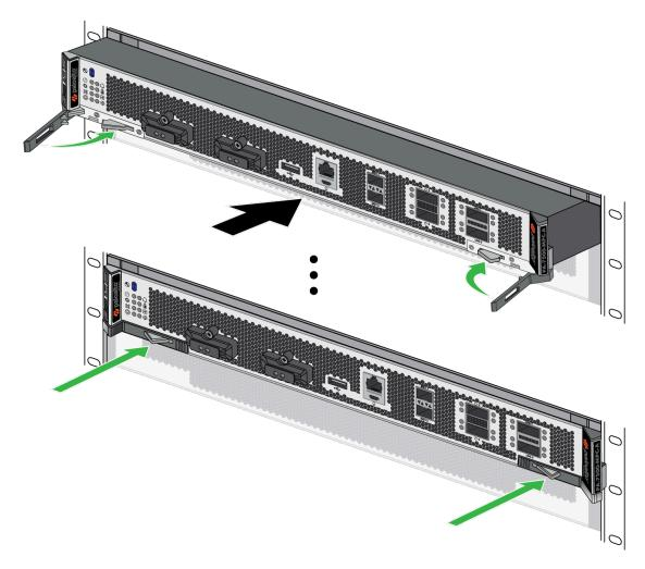
(SFC) Pull the ejector tabs away from the center and rotate the handles outwards. Then gently push the interface card into the appropriate slot until the card reaches the end of the slot.
