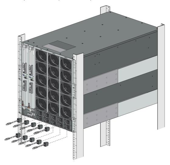
STEP 7 | Install blanks into any unused power supply slots to help maintain chassis air flow. Slide the blank into the slot until the thumb tabs click into the locked position.
