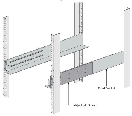
STEP 3 | Adjust the brackets to fit the depth of the equipment frame, then secure the brackets to the equipment frame with mounting screws (not provided) compatible with your equipment frame. Tighten the screws to their recommended torque value.
