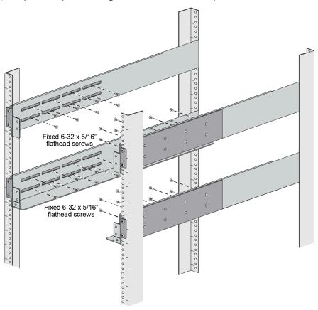
STEP 6 | Slide the PA-7500 on the brackets that were previously mounted to the equipment frame until the front mounting flanges of the PA-7500 are flush against the mounting surface of the equipment frame.
