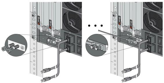
STEP 5 | Crimp a 6-AWG wire to the provided grounding lug and connect the other end to your earth ground point.
