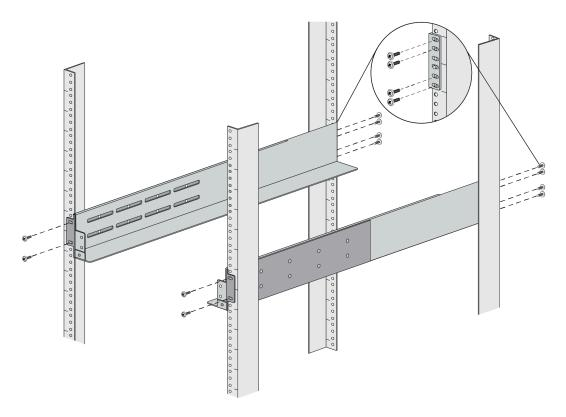
STEP 4 | Use the provided 6-32 x 5/16 flathead screws to secure the adjustable bracket to the fixed bracket. A minimum of 6 screws are required for each side.
