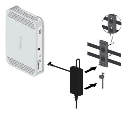
STEP 5 | After you secure the power adapter to the bracket, mount the bracket next to the firewall using wood or drywall screws as appropriate.
