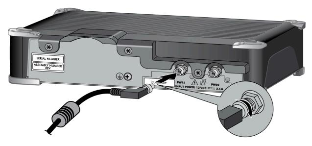
STEP 4 | Plug the connector from the power adapter into your power source. After power is connected, the firewall powers on as indicated by the green power LED next to the PWR 1 port. The front PWR LED shows green when a functioning power adapter is connected.
