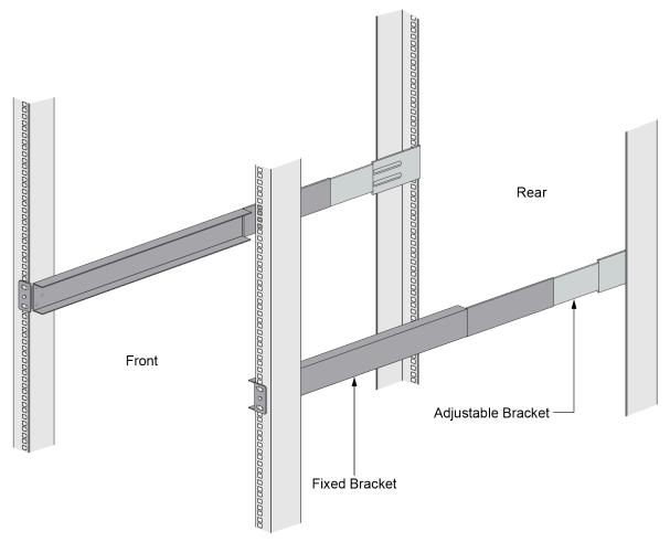
STEP 2 | Align the bottom edge of the mounting rails to the bottom of the 1 RU reserved for your firewall. Align the slotted holes in the adjustable mounting bracket to the holes on the rear of the equipment frame.
