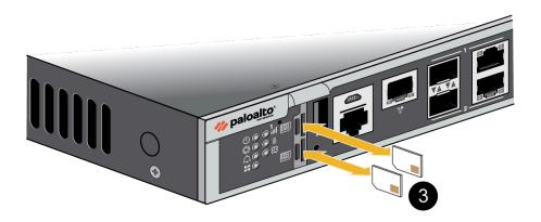
STEP 3 After inserting the SIM, place the SIM cover back onto the device and fasten the screw(s).
