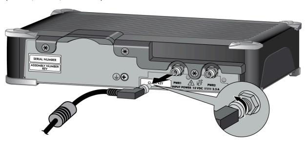
(PA-410) Unplug the failed power adapter from the AC power source and pull the power cable out of the firewall to remove it.
