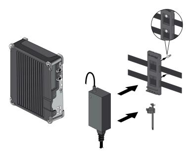
(PA-415, PA-415-5G, PA-455, PA-455-5G, and PA-445) Install the power adapter in the power adapter wall-mount bracket using the Velcro straps and cable tie. Make sure to align the cable tie with the notches in the bracket to prevent the power cord from falling out. Next, loop the two Velcro straps through the side openings on the wall mount and over the power
