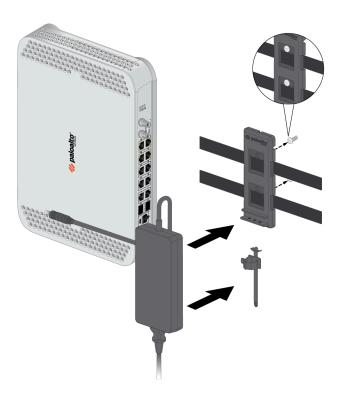
(PA-410) Install the power adapter in the power adapter wall-mount bracket using the Velcro straps and cable tie. Make sure to align the cable tie with the notches in the bracket to prevent the power cord from falling out. Next, loop the two Velcro straps through the side openings on
