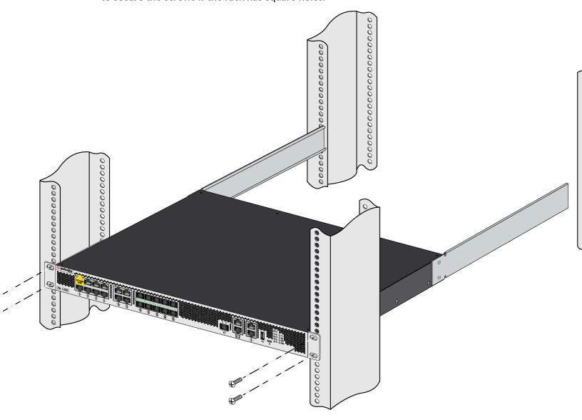
STEP 4 | Slide one back rack-mount bracket into each of the two previously installed side rack-mount rails and secure the brackets to the back rack-posts using the appropriate screws for your rack (#10-32 x 3/4" or #12-24 x 1/2") and torque to 25 in-lbs.
