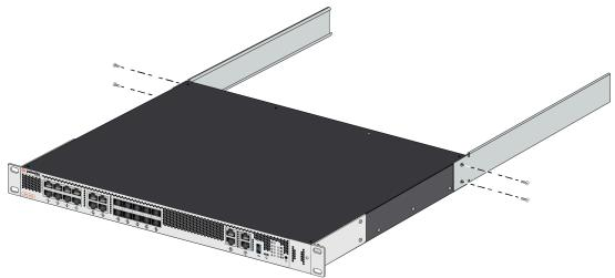
STEP 3 | Hold the device in the rack and secure the front rack-mount brackets to the front rack-posts using two screws for each bracket. Use the appropriate screws (#10-32 x 3/4" or #12-24 x
