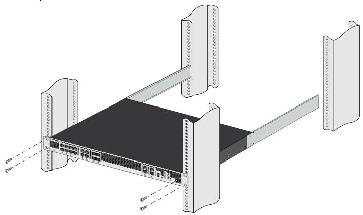
STEP 4 | Slide one back rack-mount bracket into each of the two previously installed side rack-mount rails and secure the brackets to the back rack-posts using the appropriate screws for your rack (#10-32 x 3/4" or #12-24 x 1/2") and torque to 25 in-lbs.
