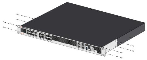
STEP 2 | Attach one rack-mount rail to each side of the device using two #6-32 x 5/16" screws for each rail and torque to 9 in-lbs.
