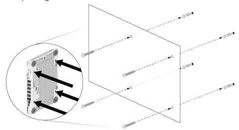
Screws and anchors are part of the wall-mount kit which is a separate kit option.
