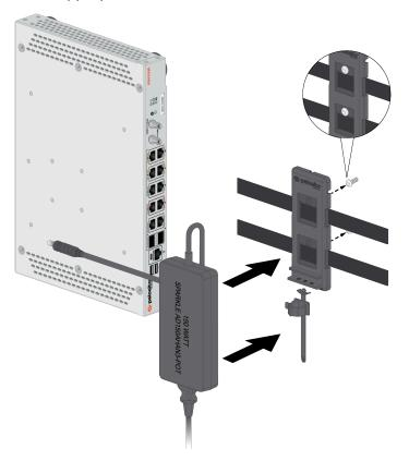
The following image shows a completed installation for an ION 3200 with a single power adapter.
