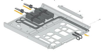
STEP 6 | Plug the power supply connector into the back of the device. Using the provided tie-wraps, bind and secure the power supply cable toward the back end of the tray using the sheet-metal lances toward the center of the tray.
