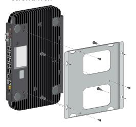
STEP 3 | Attach the wall mount to the wall using four screws that are appropriate for your wall (sheet metal and drywall inserts are included with the wall mount kit). Ensure that the side fins run vertically, as shown in the above figure.
