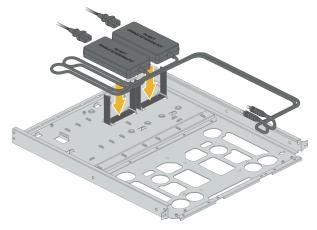
ION 3200 device comes with only one power adapter. The second power adapter as shown in the image is an optional power adapter.
