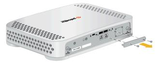
STEP 2 | Insert the nano SIM in SIM 1 or SIM 2 slot by pushing the SIM in the slot till it is locked in its position.
